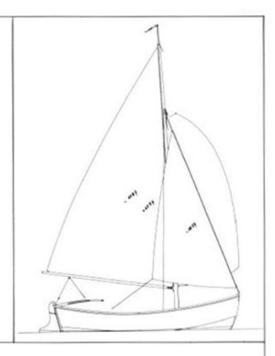
The sloop TERN is a safe, simple hard-chine dinghy, conceived as a modification to GOSLING (Plan #22) but with easier construction and more load-carrying ability. She has a jib-headed rig (64 square feet) and could carry a spinnaker. TERN will hold three children or two adults, and could be built in fiberglass or plywood.
