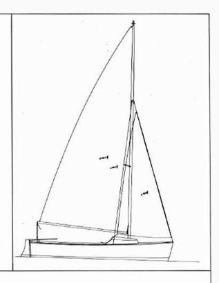
The fiberglass, jib-headed sloop SCORPION has a high aspect ratio rig and excellent windward ability. She carries four adults, could easily take an outboard motor, and can be constructed with a cuddy or half decked.
