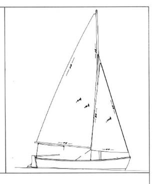
LITTLE BEAR was originally designed for Sailstar Boats of West Warwick, Rhode Island as a larger version of the SPIRIT (Plan #20). A compact fiberglass sloop, LITTLE BEAR is pretty and seaworthy — "a going little boat" — with 86 square feet of sail. She can be sailed, outboard-motored or rowed and is a good boat for sail training, daysailing, racing or frostbiting. She is so light (200 lbs) that one man can trail her, launch her and sail her, yet she has room enough for a family of four.
